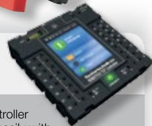
The compact ROBOTICS TXT Controller (90x90x25 mm) can be controlled easily with the color 2.4" touch display. The combined Bluetooth / WiFi RF module provides the perfect, wireless interface for numerous applications. The numerous interfaces also include a USB host port for USB sticks and other components such as the fischertechnik USB camera. Integrated Micro SD card slot allows expansion of memory capacity. Controllers can be coupled.
