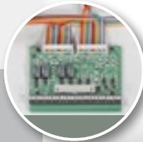
**Port:** PCB with relays to reverse polarity of motor, multi pin connector (26 pins, grid 2,54mm) and in addition PCB terminals with push in connection for all I/O
